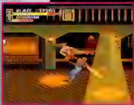
[Mega Drive] On real hardware, low-quality video output allows the pixels to blend together into a convincing transparency effect.
